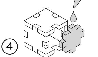
Once verified the correct assembly sequence, just add a small quantity of PVA glue on every joint.
